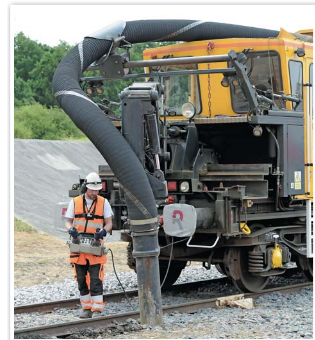
Demonstrations are a key part of the Rail Live experience. Railcare's Railvac OTM Ballast Vacuum Extraction System was at the 2018 show. CHRIS LOWNDES/RAIL.
